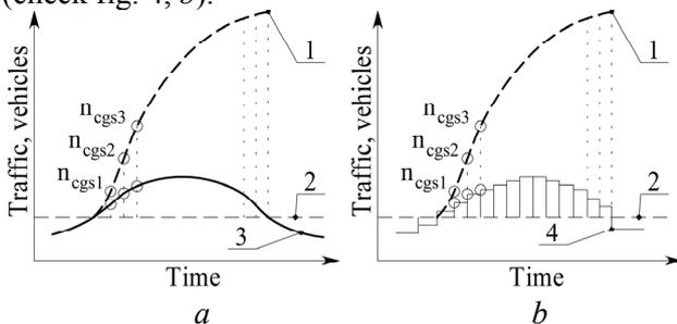
**Fig. 4.** Determination of the congestion queue length: *a* – in case the traffic intensity is changed by the function  $\lambda(t)$ ; *b* – in case of a discrete change  $\lambda$ :
