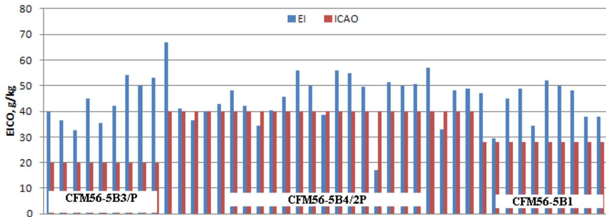
**Fig. 2.** Comparison EICO determined for CFM-5Bx engines with ICAO values for idling aircraft at European airports (London-Heathrow in 1999 and 2000, Frankfurt/Main in 2000, Vienna in 2001)
