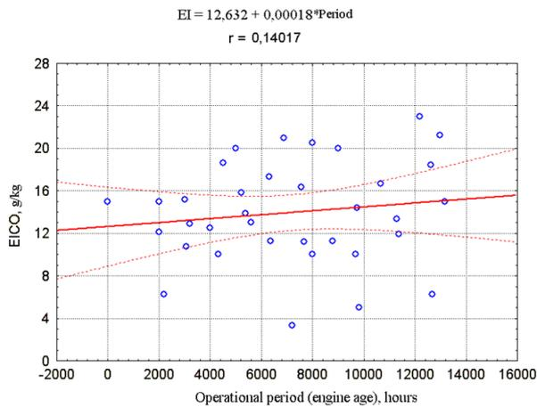
**Fig. 5.** Dependence of EICO on operation hours of CFM56-5C2/F engine of A340 (D-AIGD, D-AIGF) aircraft
