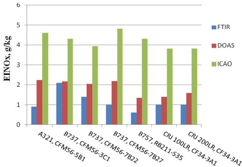
**Fig. 3.** Comparison measured EINOx by FTIR and DOAS with ICAO values during measurement campaign for idling aircraft at European airports
