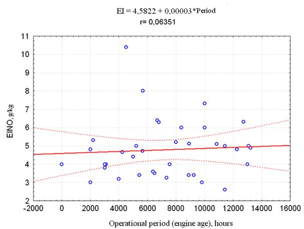
**Fig. 6.** Dependence of EINO on operation hours of CFM56-5C2/F engine of A340 aircraft (D-AIGD and D-AIGF)
