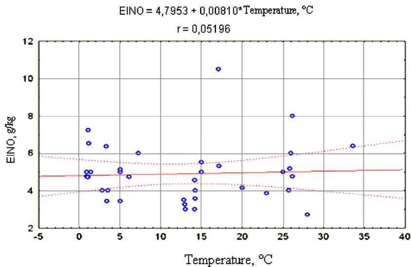
**Fig. 8.** Dependence of EINO on ambient temperature for cruise conditions of CFM56-5C2/F engine of A340 (№ 3, 4 D-AIGF, D-AIGD) aircraft
