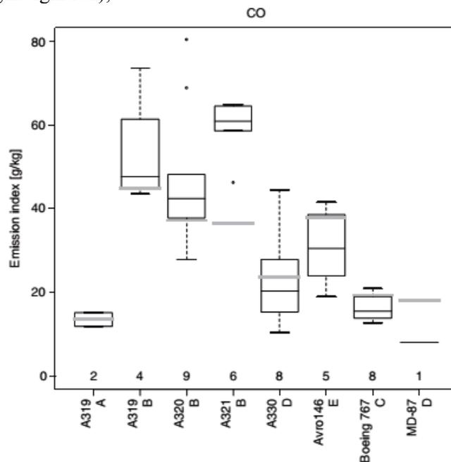
**Fig. 4.** Comparison measured EICO (a black vertical bar with horizontal lines of minimum, median and maximum meaning) with ICAO values (a grey horizontal bar) during measurement campaign for idling aircraft at Zurich airport. The letter adjacent to each aircraft type denotes a specific class of engines
