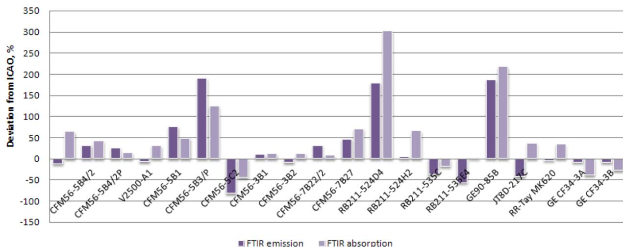
**Fig. 1.** Comparison measured EICO by FTIR emission and absorption spectrometry during measurement campaign for idling aircraft at European airports (London-Heathrow in 1999 and 2000, Frankfurt/Main in 2000, Vienna in 2001)
