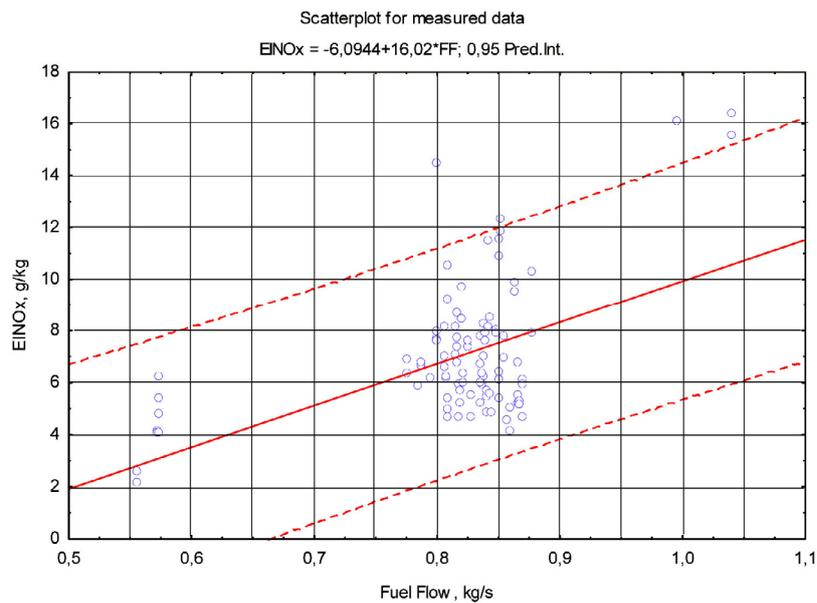
**Fig. 9.** Dependence of EINO<sub>x</sub> on measured Fuel Flow for cruise conditions of CFM56-5C2/F engine of A340 (№ 3, 4 D-AIGF, D-AIGD) aircraft
