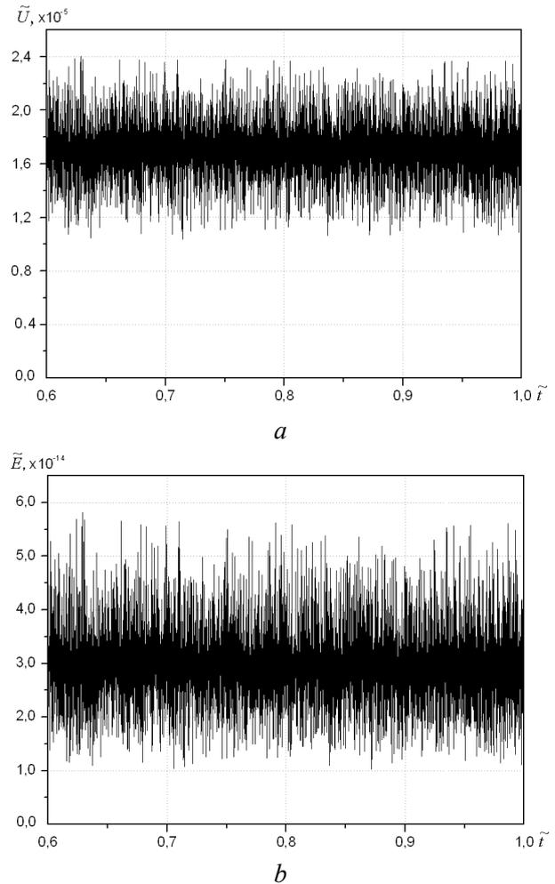
**Fig. 2.** Graphs of the variation of the resulting AE signals amplitude (a) and energy (b) over time in relative units during machining of CM. Simulation parameters:  $\tilde{\chi} = 20$ ,  $\Delta \tilde{t}_j = 0,1$ ;  $\tilde{\tau}_0 = 10^{-7}$ . The value  $\tilde{\delta}$  varies in the range of values from 0 to 0.16. Value  $\Delta t_k = 0,0001$
