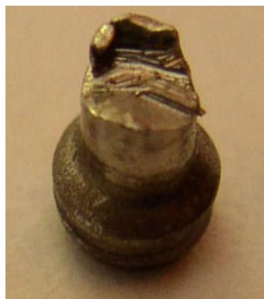
**Fig. 6.** Fatigue destruction of rod neck
