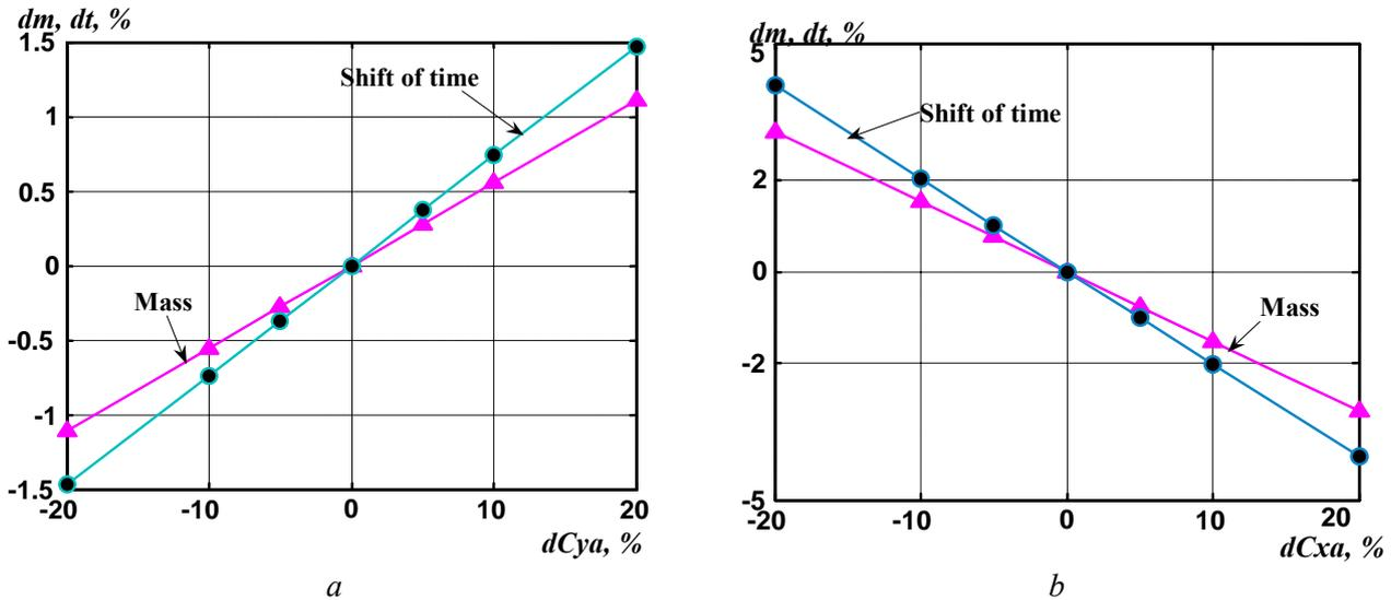
Fig. 5. Influence of aerodynamic coefficients designation error on initial time and mass estimation shift: *a* – designation error of  $c_{ya}$  coefficient; *b* – designation error of  $c_{xa}$  coefficient
