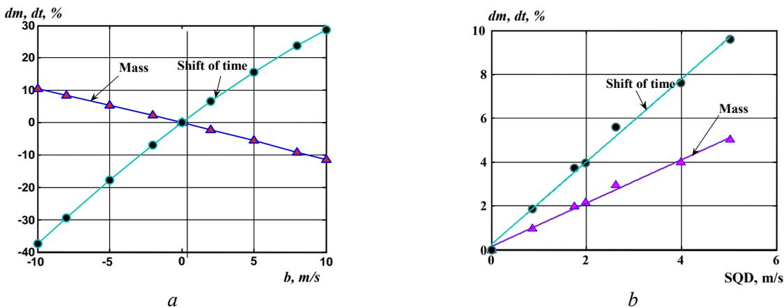
**Fig. 3.** Influence of take-off run speed error value on initial time and mass estimation shift: *a* – systematic error; *b* – random error
