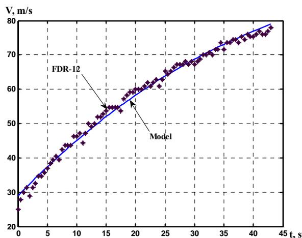
Fig. 6. An-24RV speed variation during take-off run
