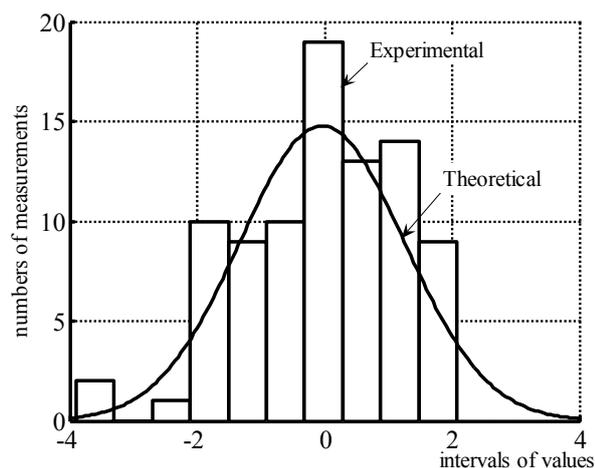
Fig. 7. Distribution density of take-off run speed rests and their approximation using normal distribution law
