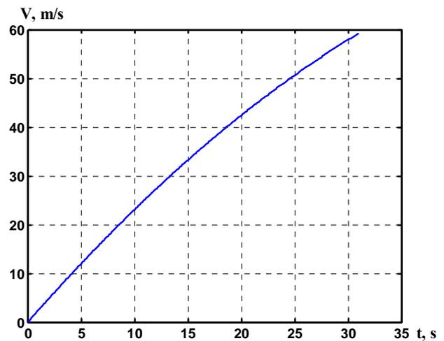
Fig. 2. Variation of An-24 take-off run speed with mass of 21000 kg.
