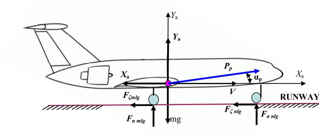
Fig. 1. Forces that act on an airplane during take-off run
