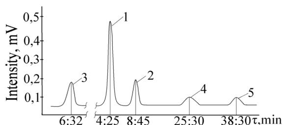
**Fig. 3.** Chromatographic analysis of isovaleric aldehyde electroreduction products on Cd – electrode in sulfuric acid-, water-alcohol solution:
