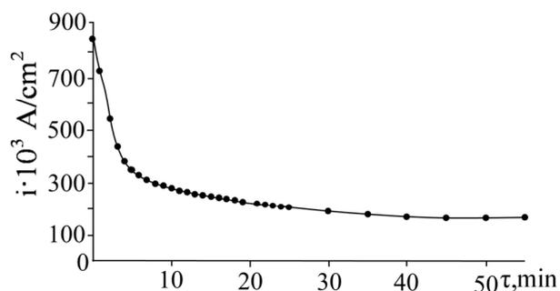
**Fig. 2.** The dependence of the limiting current density of isovaleric aldehyde recovery in sulfuric acid-water-alcohol solution
