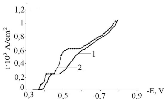
**Fig. 1.** Polarization curves of cadmium:
