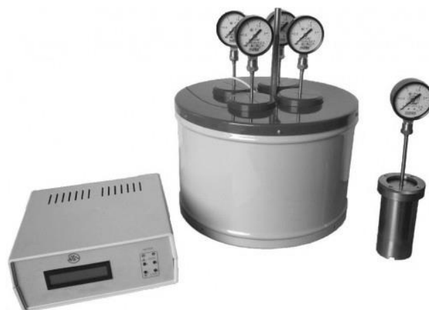
Fig. 2. Device for studying the oxidative stability of fuels and lubricants TCPT-2M
