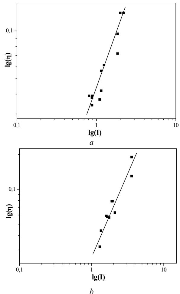
**Fig. 1.** Diffraction efficiency dependence ( $\eta$ ) on the value of the laser radiation intensity ( $I$ ) for the coloured samples of LLC-HD<sup>2+</sup>2Br<sup>-</sup> (a) and LLC-CED<sup>2+</sup>2Cl<sup>-</sup> (b)
