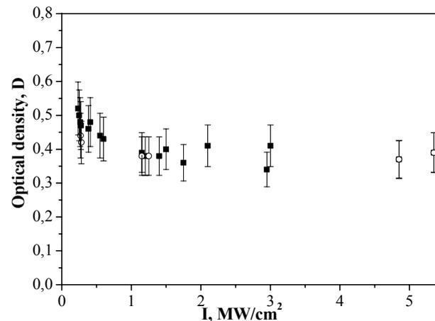
**Fig. 2.** Optical density dependence ( $D$ ) on the value of the laser radiation intensity ( $I$ ) for LLC-viologen samples: ■ corresponds to the measurements at an intensity increase; ○ corresponds to the measurements at an intensity decrease
