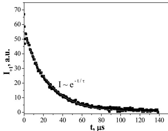
**Fig.3.** Kinetics of gratings erasing in a microsecond time range for LLC-viologen samples
