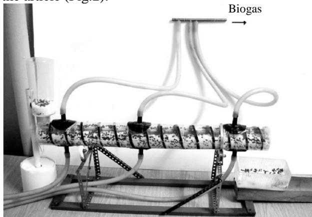
**Fig. 2.** Demonstration model of continuously working screw methane-tank
