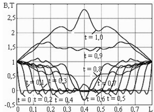
Fig. 4. The field distribution along the middle line of the core cross section ( $Re_M = 5, \beta = 1$ ).
