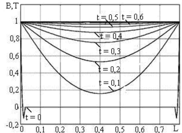
Fig. 5. Diffusion process of the field setting up in the cross section of core for  $Re_M = 5, \beta = 0,01$ .
