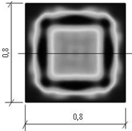
Fig.3 Two-dimensional picture of field in the cross section of core for meanings of parameters  $Re_M = 1, \beta = 1$ .
