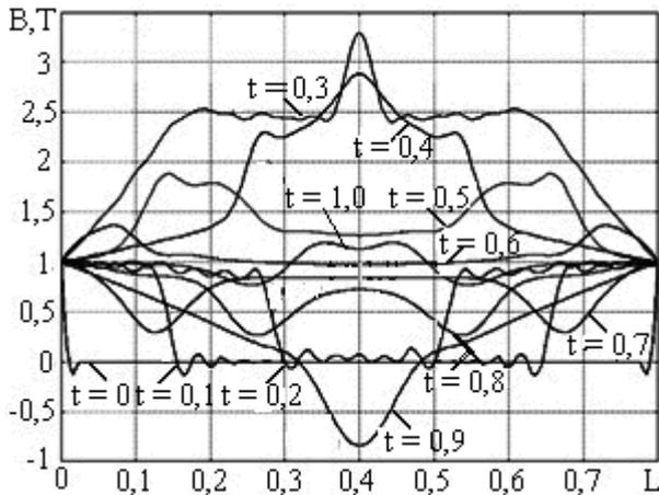
Fig.2. Distribution of field along the middle line of the core cross section ( $Re_M = 1, \beta = 0,5$ ).
