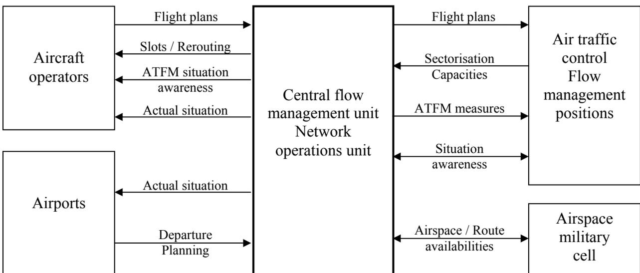
Fig. 2. Operational Structure with CFMU Network Operations Unit
