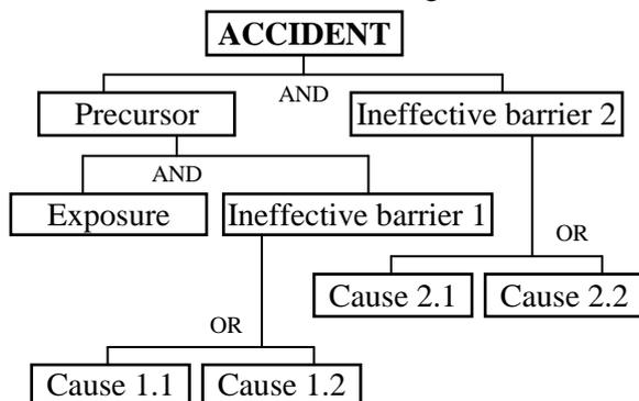
Fig. 4. Schematic fault tree structure
