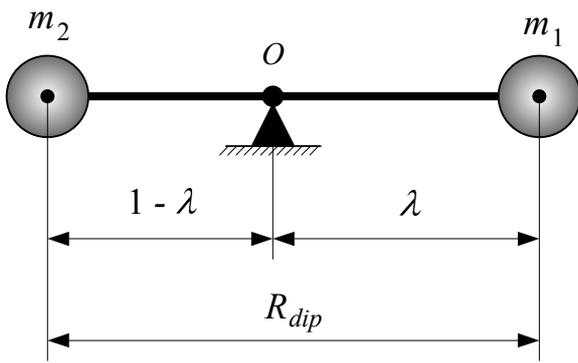
Fig. 4. The kinematic scheme of the virtual meter of "dipole" type at experiment 1
