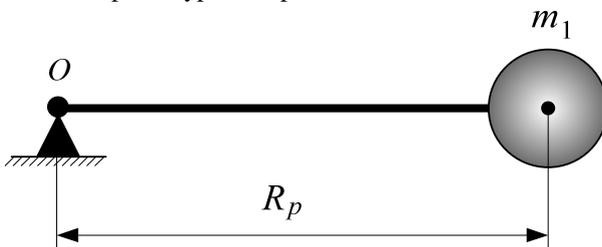
Fig. 6. The kinematic scheme of the virtual meter of "pendulum" type at experiment 3
