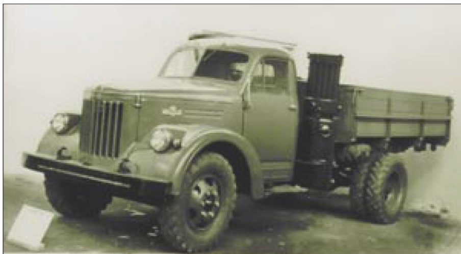
Fig. 1. The “Uralzis” WWII era Soviet pyrolysis powered truck
