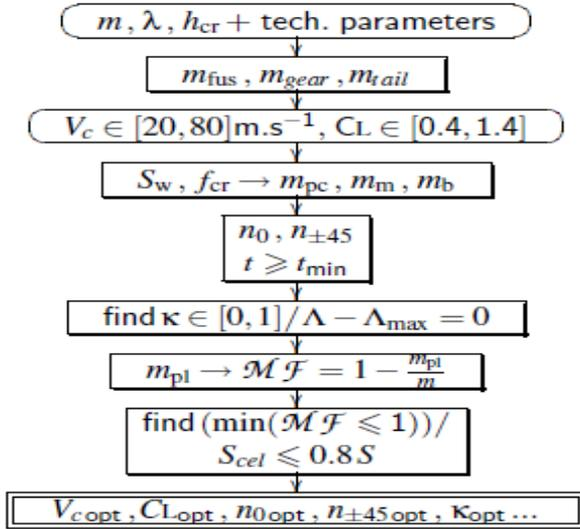
Fig.3. Diagram of the algorithm for calculating the optimized UAV
