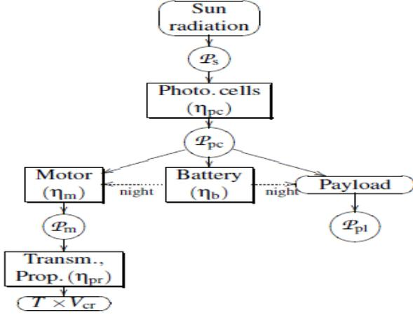
Fig.1. Block diagram of power distribution
