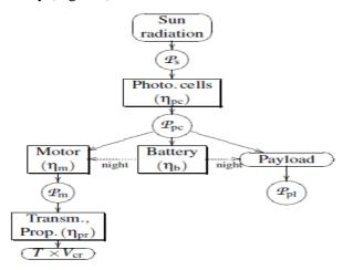
Fig.1. Block diagram of power distribution
