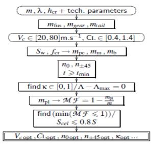
Fig.3. Diagram of the algorithm for calculating the optimized UAV
