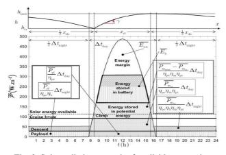
Fig. 2. Solar radiation per unit of available space, time and energy distribution for engines, battery and payload battery
