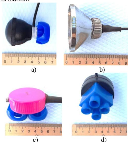
Fig. 3. Receivers of acoustic information as constitutive element of the UAV-system for remote diagnostics and monitoring "Trembita-Corona UAV NAU":
