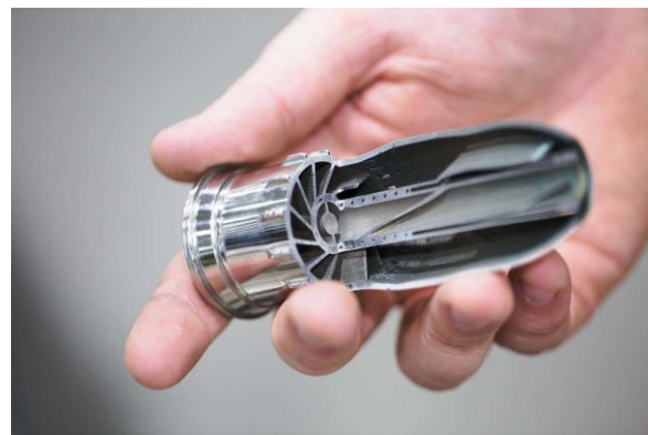
Fig. 2. Fuel injector CFM LEAP, manufactured by additive technology
