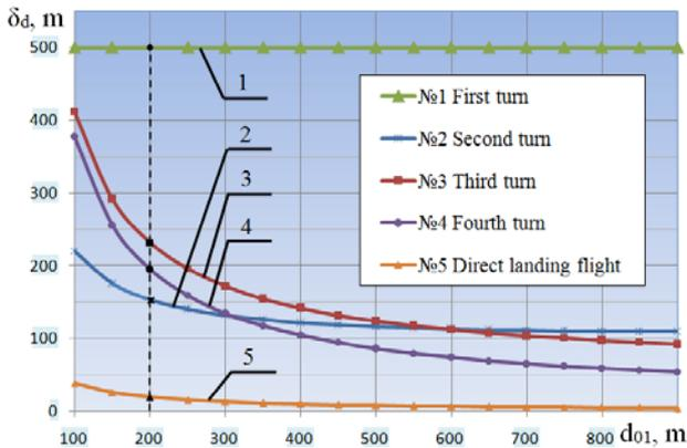
Fig. 4. Dependency graph of the error determining, by the MPLS system, the aircraft deviation from the center line of the runway at turns and on the aircraft direct flight trajectory  $\delta_d$  versus the distance between its GE components  $d_{01}$
