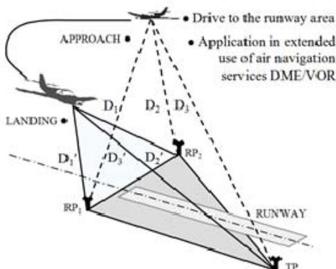
Fig. 1. The principle of MPLS operation
