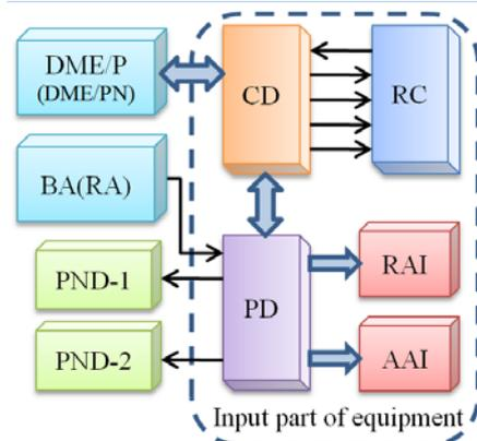
Fig. 2. Scheme electrical structural MPLS airborne equipment
