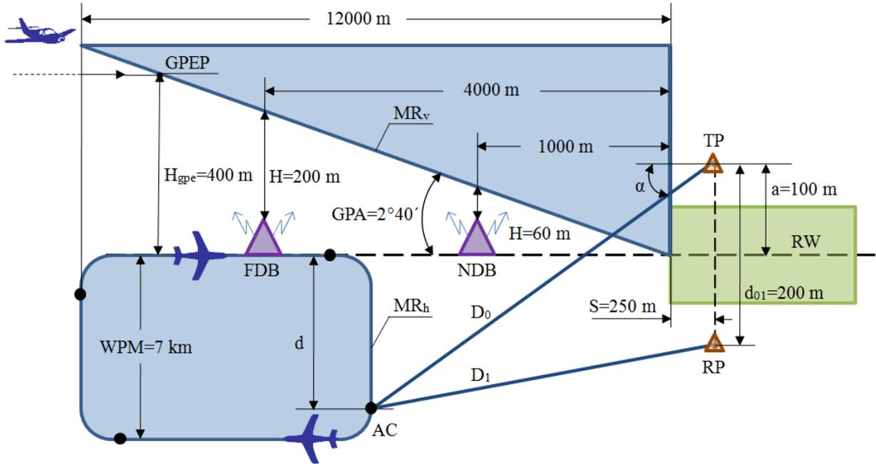
Fig. 3. The basic geometric correlation between the placement of beacons and runway to the estimation of errors in determining AL during its pre-landing maneuvering
