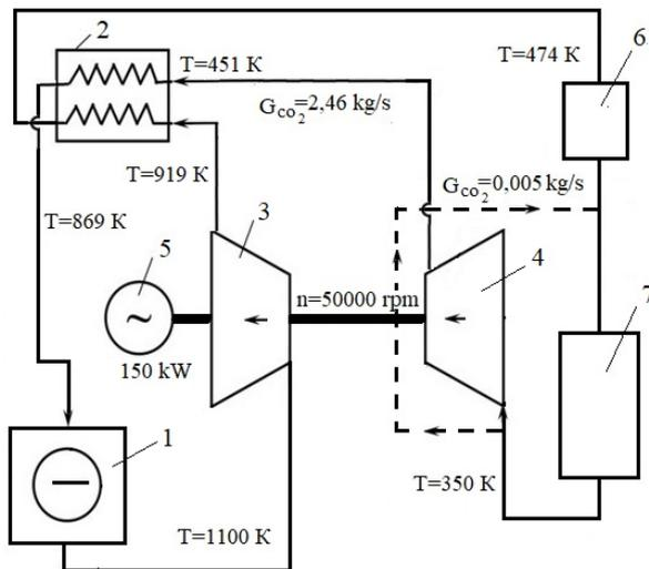
Fig. 3. The scheme of a closed-cycle gas turbine plant: 1-compressor; 2- turbine; 3- electric generator; 4-regenerator; 5-gas heater; 6 - gas cooler; 7- object for conditioning
