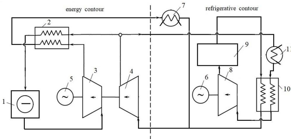
Fig. 1. Scheme of closed cycle gas turbine plant with parallel connected energy and refrigerative parts:
