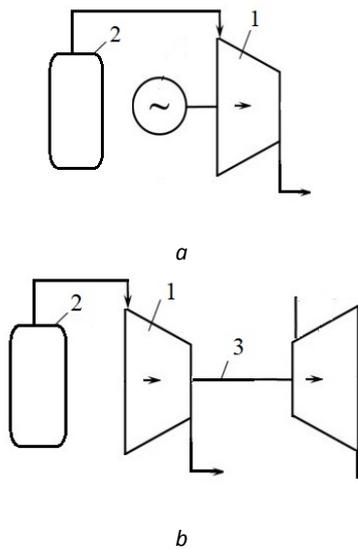
Fig. 2. Working fluid leakage compensation system: 1- booster compressor; 2- feed vessel
