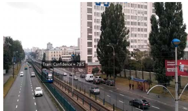
Fig. 3. Detected tram and detection scores for frame 242
