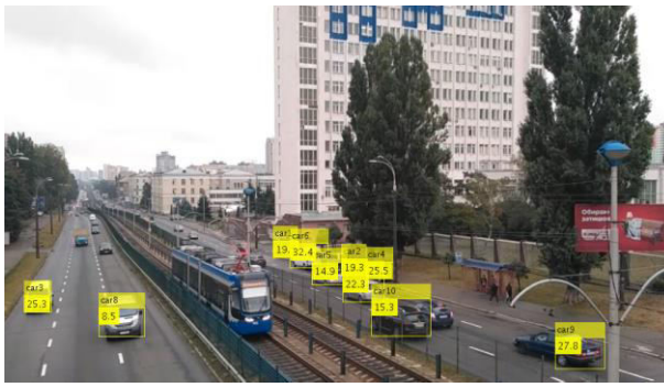
Fig. 4. Detected cars and detection scores for frame 342
