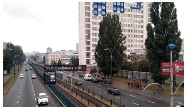
Fig. 2. Detected tram and detection scores for frame 262
