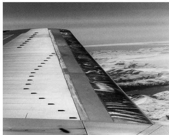
Fig. 3. VRTs installed in front of an aileron and the separation zone (Boeing 737)
