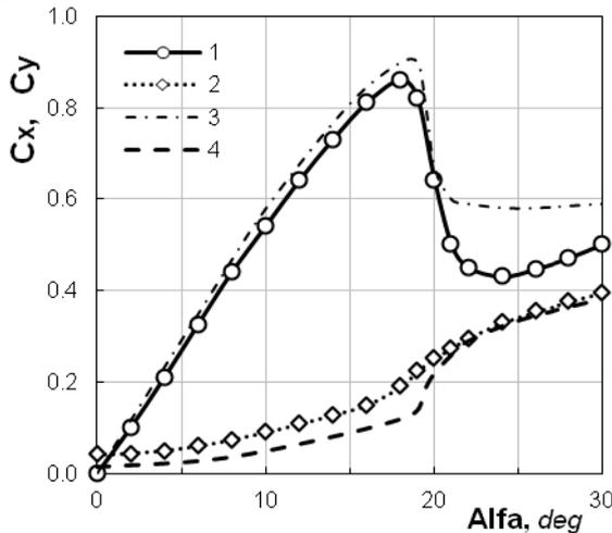
Fig. 2. Lift  $C_y$  (1,3) and drag  $C_x$  (2,4) coefficients of the wing with the elongation  $\lambda = 1.5$ , depending on the angle of attack in the steady flow: 1,2 – present work, 3,4 – [12, 13]
