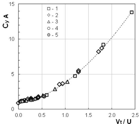
Fig. 3. Amplitude of oscillations of the wing lift coefficient  $C_{yA}$  for different values of the frequency  $f$  and the flow velocity  $U$  with amplitude  $\beta = 30^\circ$ , depending on the parameter  $V_t/U$ . 1 –  $U = 0.22$  m/s; 2 –  $0.31$  m/s; 3 –  $0.5$  m/s; 4 –  $1.0$  m/s; 5 –  $1.5$  m/s, respectively oscillation frequencies  $f = 0.31, 0.5, 1.0, 1.5$  и  $2.0$  Hz.
