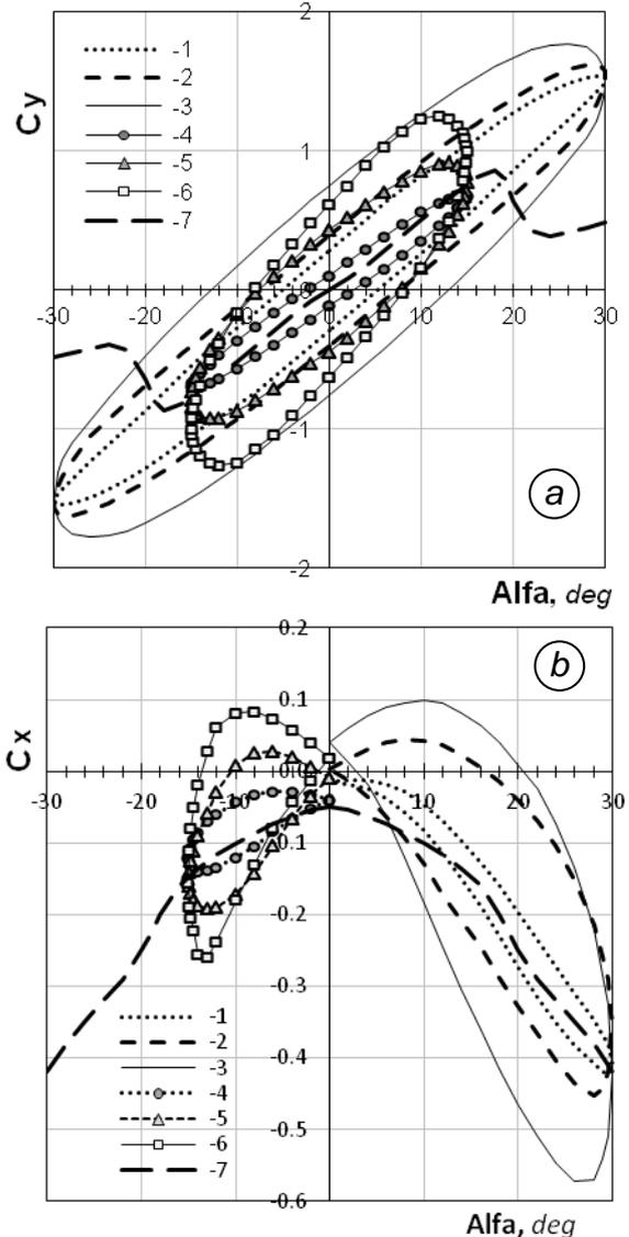
Fig. 4. Variation of transverse  $C_y$  (a) and longitudinal  $C_x$  (b) coefficients of hydrodynamic force component within a one period of oscillation as a function of the instantaneous value of the pitch angle  $\alpha$ , at different frequencies and amplitudes of the wing oscillations.
