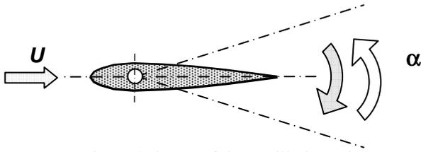
Fig. 1. Scheme of the oscillating wing
