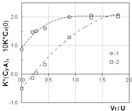
Fig. 5. Maximum values of the lift coefficient  $C_{yA}$  (1) and longitudinal force (drag-thrust) during passing a zero pitch angle ( $\alpha = 0$ )  $C_x(0)$  (2) for different values of the wing oscillation frequency ( $f = 0.0, 0.23, 0.31, 0.5, 1.0, 1.5, 2.1$  Hz), at flow velocity  $U = 0.31$  m / s, depending on the parameter  $V_t / U$ .
