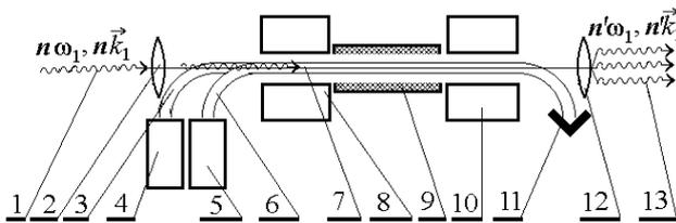
Fig. 2. Simplest variant of design scheme of the klystron-TSFEL-amplifier:
