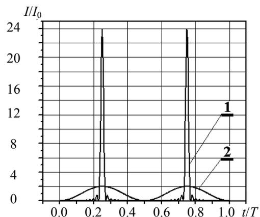
Fig. 3. Dependency of the normalized signal intensity  $I/I_0$  on the normalized duration of the femto-second wave packages  $t/T$ :
