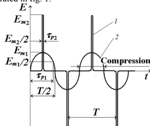
Fig. 1. The method of compression of femto-second wave packages:
