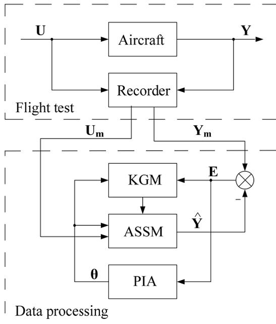
Fig. 1. The block diagram of the identification algorithm
