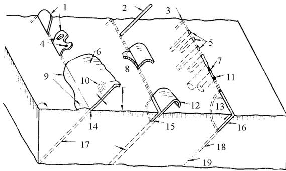
Fig. 1. Persistent slip band (PSB) formation in plastic metals:
