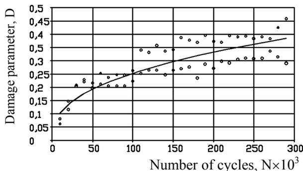
Fig. 4. The dependence of damage parameter “D” on the number of load cycles
