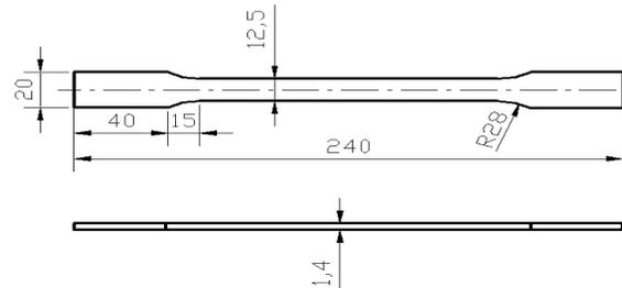
Fig. 3. Specimen for static loads
