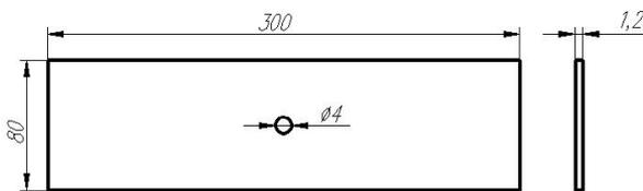
Fig. 2. Specimen for fatigue test
