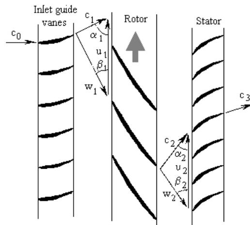
Fig. 2. The velocity diagrams for compressor stage
