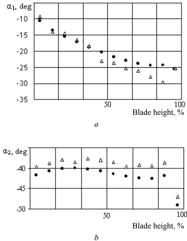
Fig. 4. Fluid angles in blade row gap along the blade height from hub to blade tips before optimization (●) and after optimization (Δ):
