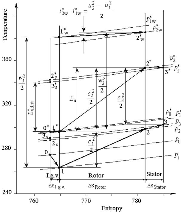
Fig. 3.  $T$ - $s$  diagram of gas compression process for the compressor stage
