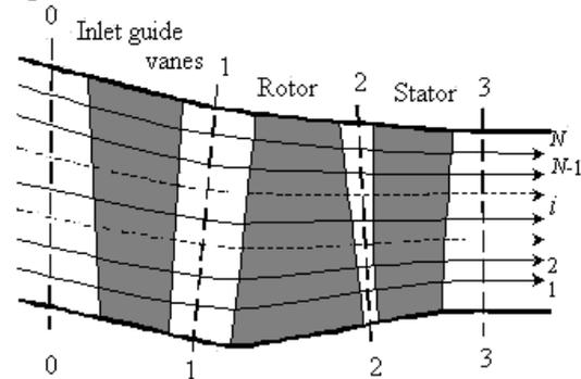
Fig. 1. Flow path for compressor stage
