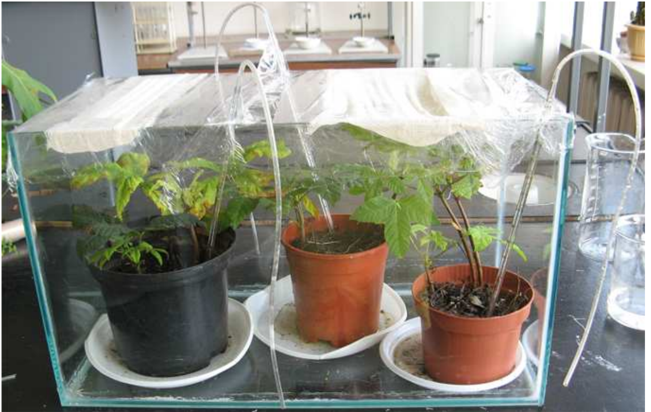
Fig. 7. One-year old horse-chestnut trees were placed in a glass aquarium for creation of isolated conditions with possibility of watering through tubes
