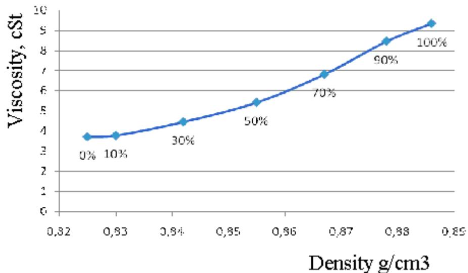
**Fig. 10. Relationship between viscosity and density for the mixtures of DF with MERO at different ratios**
