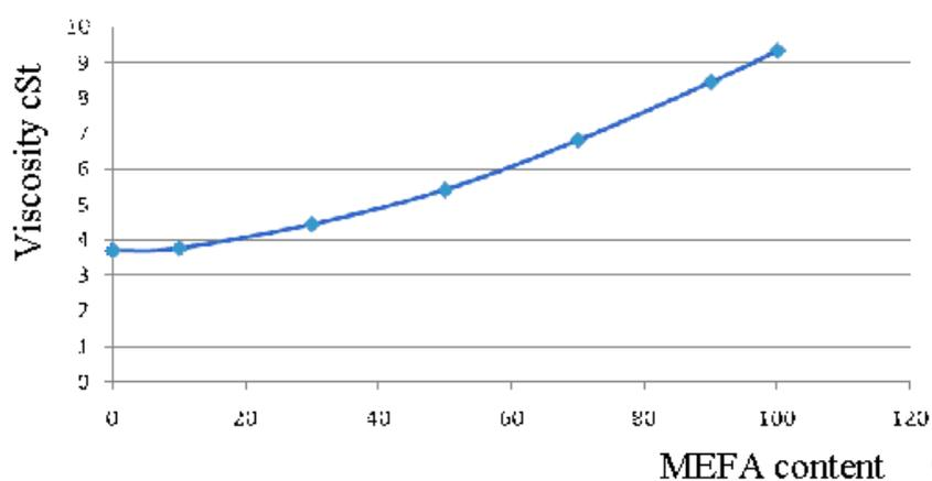
**Fig. 6. Viscosity of MERO mixtures with DF at different content of MERO (0, 10, 30, 50, 70, 90, 100 % at.)**
