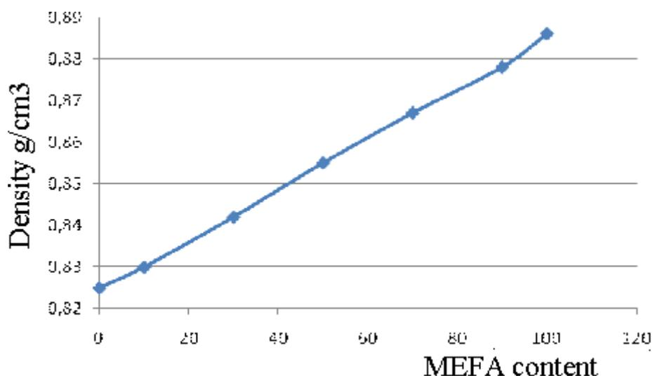
Fig. 7. Dependence of density of mixture of mineral DF with MERO from content of MERO at temperature 20,5 °C
