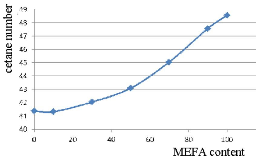
**Fig. 8. Growth of cetane number at increase of content of biodiesel in a fuel mixture**
