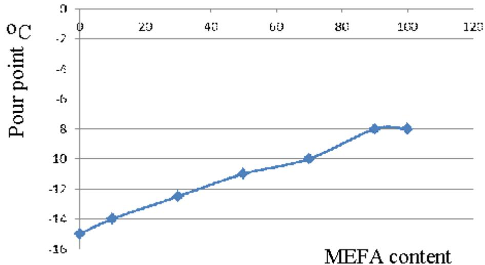
**Fig. 9. Temperature of freezing of MERO mixtures with DF at different content of MERO (0, 10, 30, 50, 70, 90, 100 % )**
