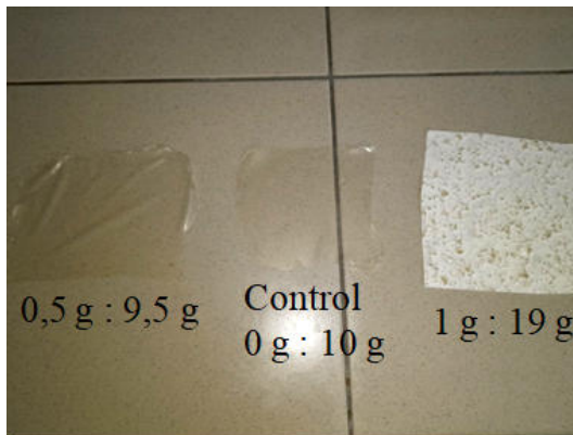
Fig. 2. Final bioplastics after 4 days drying in the thermostat (xanthan, g : starch, g)
