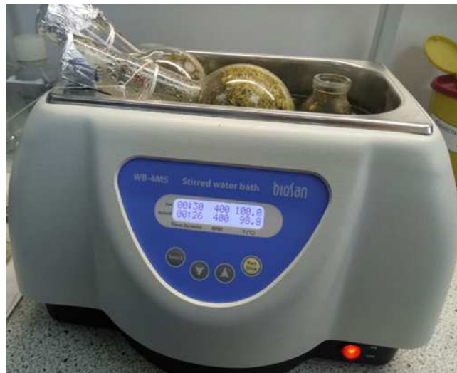
Fig. 3. Keep of extracts in a water bath (water bath-thermostat with stirring WB-4MS)
