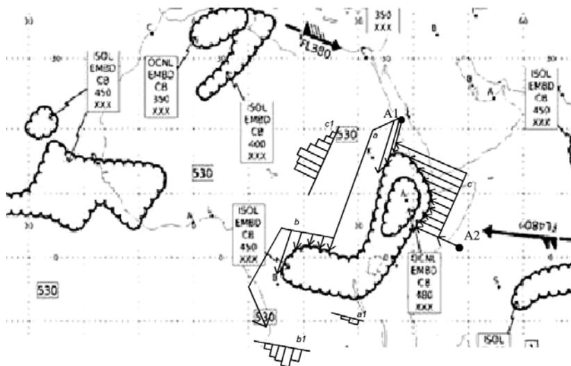
Fig. 2. Reconstruction of the dangerous phenomena area using the information from two mobile sensors-aircrafts
