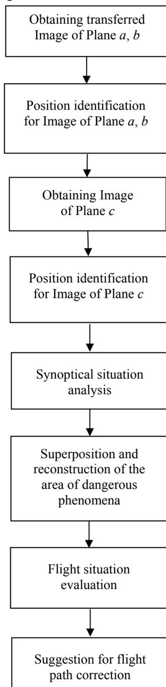
Fig. 3. Simplified order of information processing by automated onboard information system for operative flight path correction
