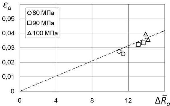
Fig. 11. The surface plastic deformation versus surface roughness relation (before 0,5 mm fatigue crack initiation).
