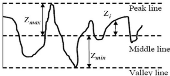
Fig. 2.  $R_a$  estimation along the line
