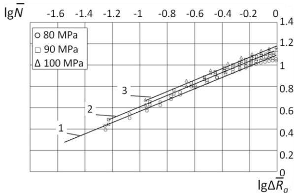
Fig. 5. Roughness increment change due to relative number of cycles spent in the 0,5 mm crack formation for different applied stress levels:  $\sigma_m$ : 1 — 80 MPa; 2 — 90 MPa; 3 — 100 MPa
