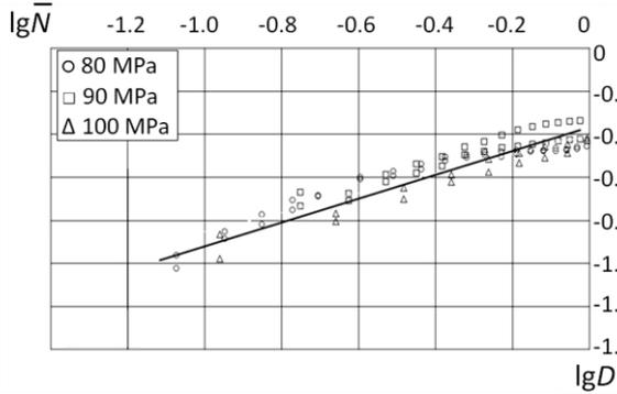
Fig. 4.  $DR$  saturation change due to relative number of cycles spent in the 0,5 mm crack formation for different stresses levels  $\sigma_m$
