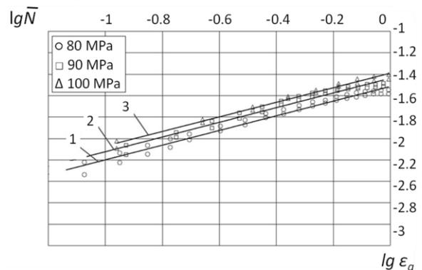
Fig. 7. Plastic deformation changes due to relative number of cycles spent in the 0,5 mm crack formation for different applied stress levels:  $\sigma_m$ : 1 — 80 MPa; 2 — 90 MPa; 3 — 100 MPa
