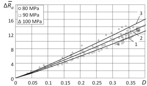
Fig. 6. Roughness increment change due to relative number of cycles spent in the 0,5 mm crack formation for different applied stress levels:  $\sigma_m$ : 1 — 80 MPa; 2 — 90 MPa; 3 — 100 MPa
