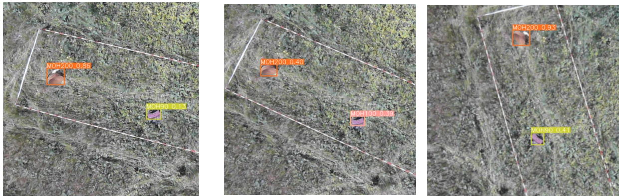
Fig. 4. Detection of MOH90 and MOH200 on the image similar to training dataset rotating the image. The result shows that orientation matters for landmines of arbitrary shape
