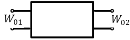
Fig. 1. Quadripole with communication lines
