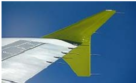
Fig. 1. The AT winglet wingtip of the Airbus A319
