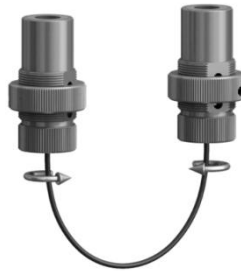
Fig.12. Wire specimen in the spindles of rotary bending machine [15]
