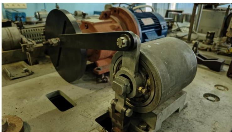
Fig. 7 – A photo of the developed installation for laboratory resource tests of aviation spherical sliding bearings.
