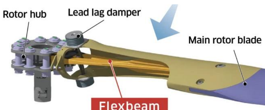
Figure 1. Bearingless rotor system design
