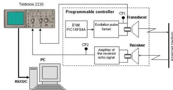
Fig. 4. Block diagram of the experimental setup
