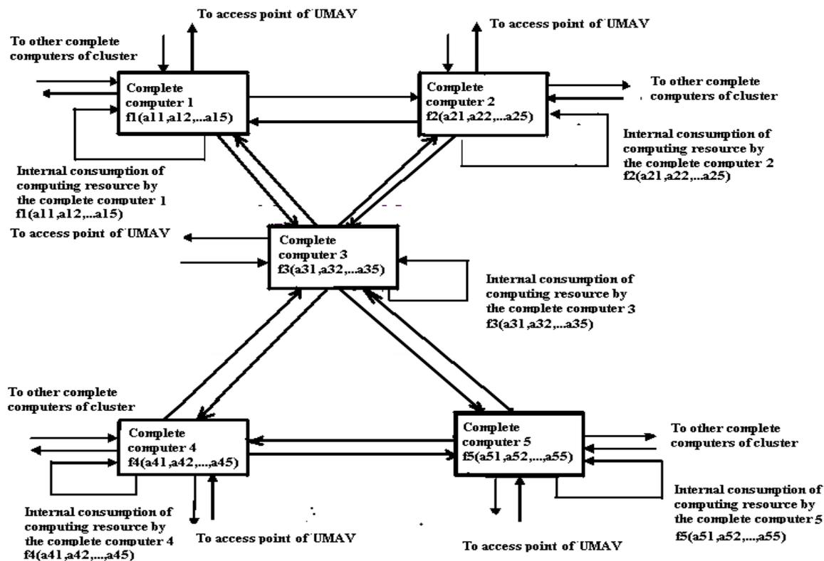
Fig. 2. Fully connected cluster with five complete computers
