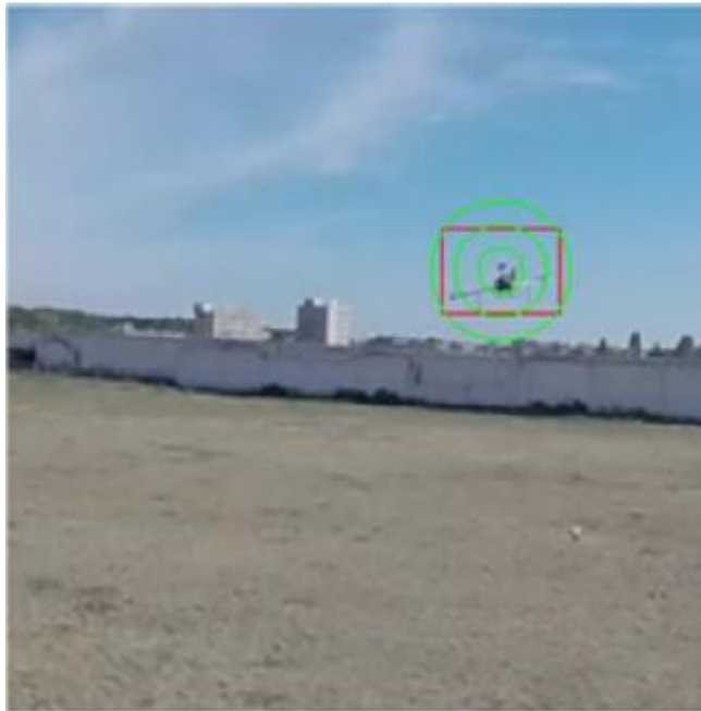
Fig. 3. Video fragment of moving object isolation in a sequence of video frames. Red rectangle indicates a moving object; green circles marked the center of object
