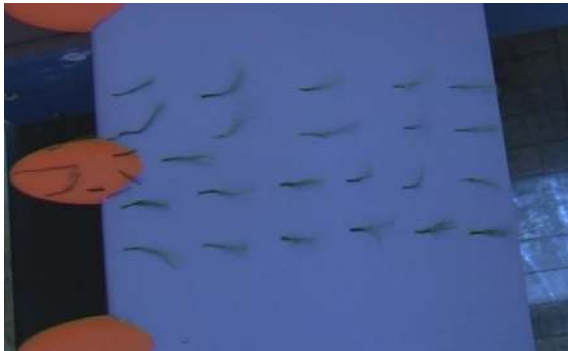
Fig. 5. Representation of the flow around the upper surface of the airfoil with vortex generators during the transition of the angle of attack to supercritical values using the silkworm method
