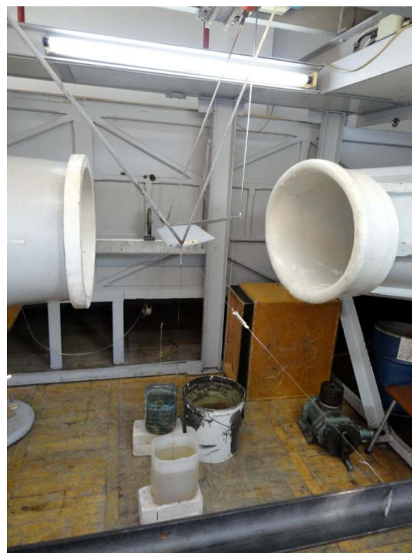
Fig. 1. The blowing model during tests on aerodynamic balance in the wind tunnel
