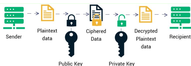
Fig. 1. Scheme of cryptographic encryption of data transmission
