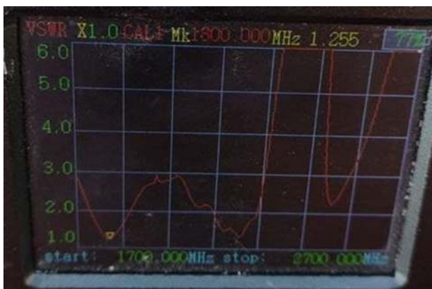
Fig. 4. The graph of dependence frequency – VSWR (Voltage Standing Wave Ratio) (Port1)
