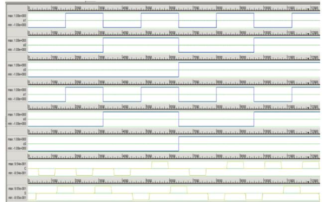
Fig. 4. Simulation of the time characteristics of a full one-bit adder on a five-inputs ME
