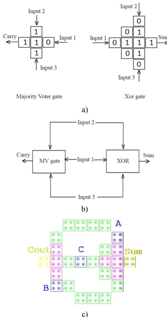
Fig. 2. Block diagram of one bit four adder: (a) is the majority voter element and XOR; (b) is the block-shart; (c) is the QSA proposed circuit
