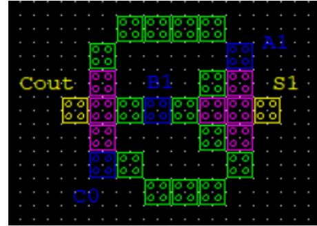
Fig. 3. Project of a complete one-bit adder on a five-inputs ME
