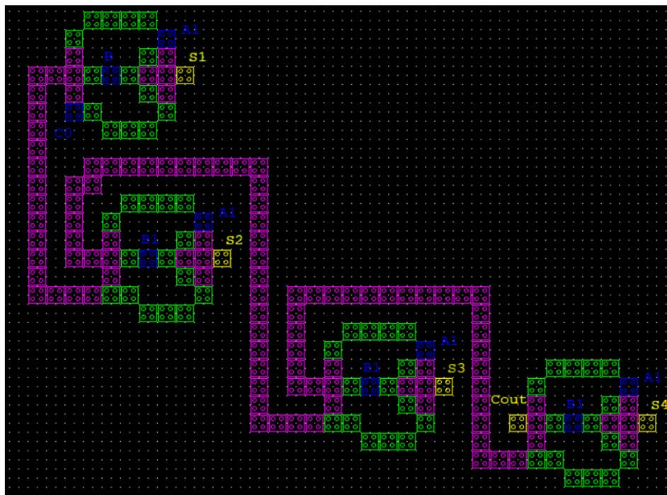
Fig. 5. The result of designing a nanocircuit of a four-bit adder
