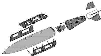
Fig. 1. Hinged set of guidance of a controlled fire-extinguishing bomb
