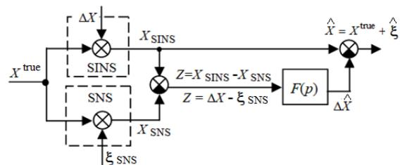
Fig. 2. Block diagram of the compensation method
