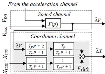
Fig. 4. Structure of the dynamic filter
