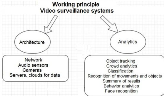
Fig. 2. Components and functionality of the video surveillance system
