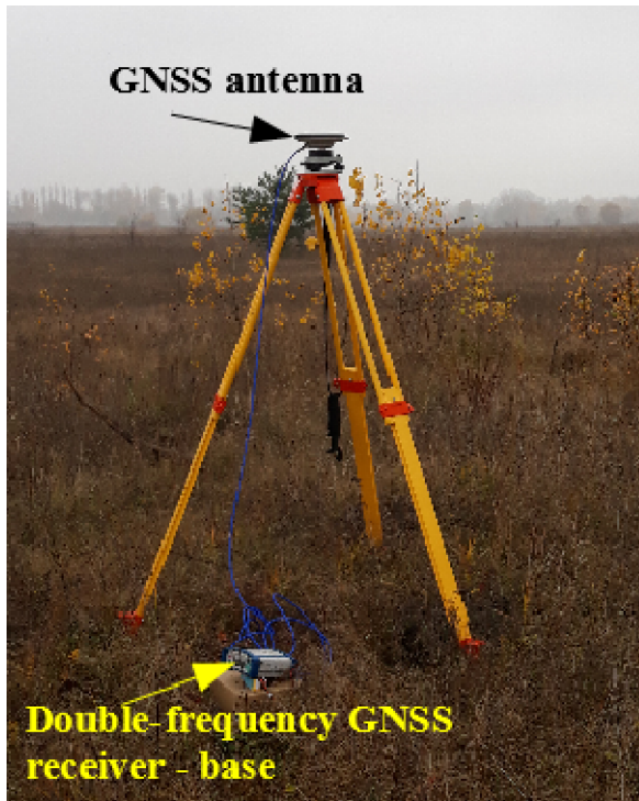
Fig. 3. Photo of GNSS equipment used for construction in post-processing of the reference trajectory: antenna and double-frequency receiver
