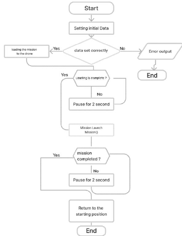
Fig. 6. Structural diagram of mission initialization
