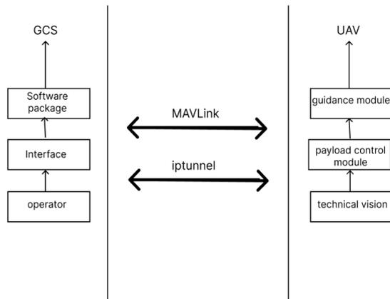
Fig. 1. Functional diagram of the UAV control subsystem
